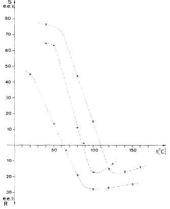
Fig. 1. Asymmetric hydroformylation of styrene in the presence of  $PtCl(SnCl_3)(BDPP)$  in toluene (+):  $PtCl_2(BDPP) + SnF_2$  in toluene (×) and  $PtCl_2(BDPP) + SnCl_2$  in dichloromethane ( $\odot$ ).
